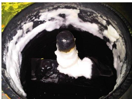
Figure 1. Black colorant in tinting machine, contaminated with mold and bacteria growth.
